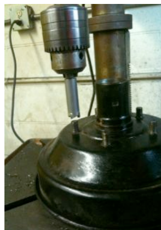
Drill press set up for stud removal
