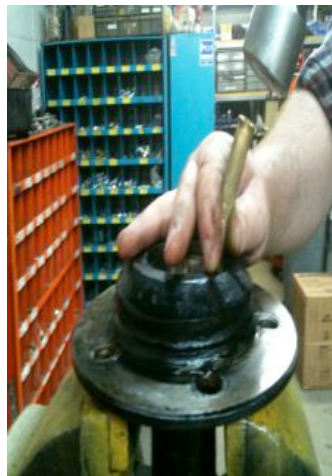
Removing the outside bearing race
