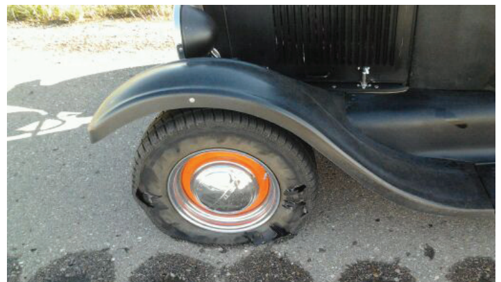
Blow out on the highway: excellent tread, aged out with rotten valve stem and sidewall.
